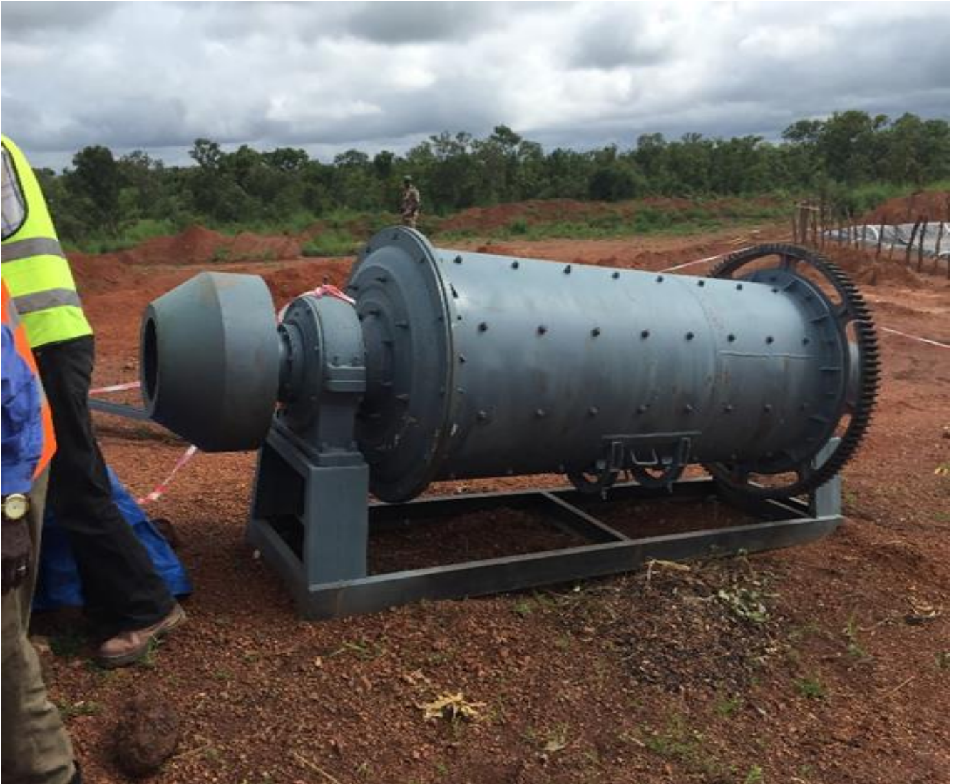
Picture 2 – Five tonnes per hour (“tph”) ball mill
